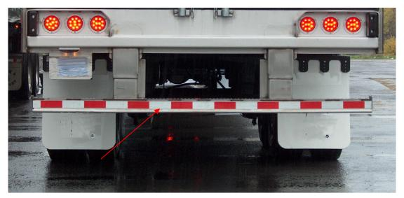
Figure 26: Example of rear underride guard
