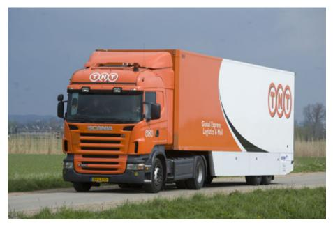
Figure 28: Example of rigid, continuous, flush fairing/side guard
