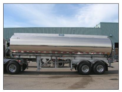
Figure 9: Sideguards installed on a Canadian operated tanker trailer
