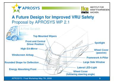
Figure 20: Future vehicle design for improved VRU safety [27]
