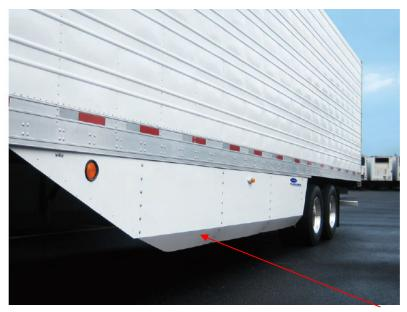
Figure 23: Example of belly fairing
