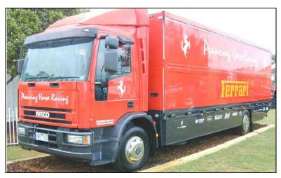
Figure 8: Example of bodywork that fulfills the sideguard regulation requirements [3]
