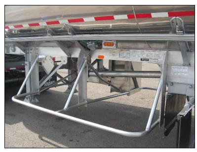
Figure 10: Close-up of a sideguard installed on a Canadian operated tanker trailer
