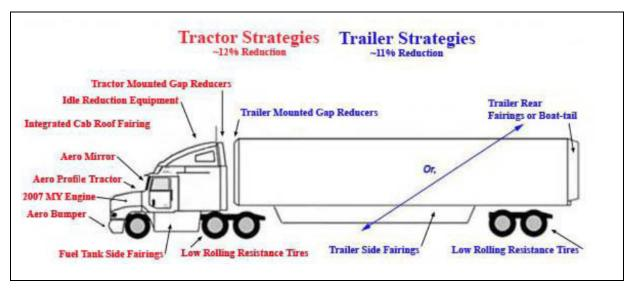
Figure 22: Examples of aerodynamic add on devices
