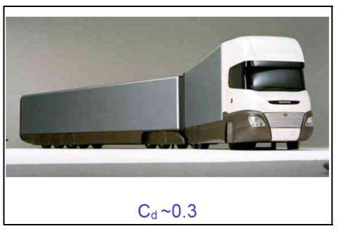
Figure 30: Example of complete aero package
