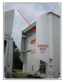
Figure 24: Example of gap fairing mounted to van semi-trailer
