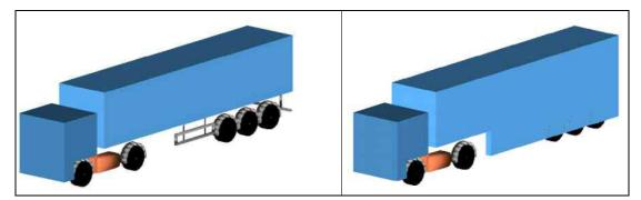
Figure 19: HGV models equipped with rail type (left) and smooth (right) sideguards [12]
