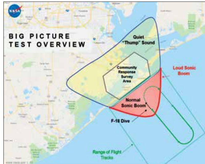
Above: The QSF18 Test over Galveston, TX. Source: NASA
