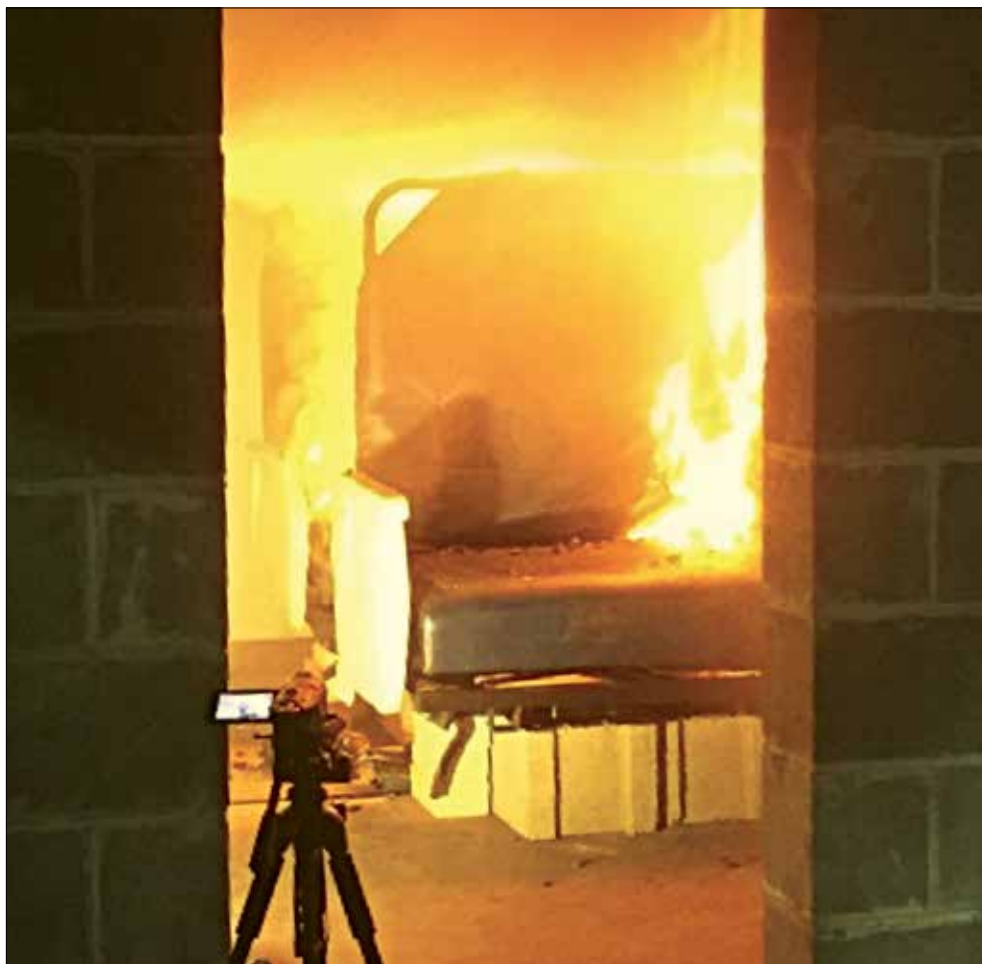
Volpe Center engineers took heat measurements during a fire test of a passenger rail car seat at the SGS Govmark testing facility in Farmingdale, New York. (Source: Volpe Center/Mark Gentile)
