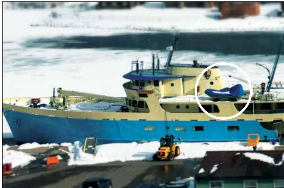
Ranger III with new rescue boat (under blue cover) and davit installed on boat deck. (Source: U.S. DOT Volpe Center)
