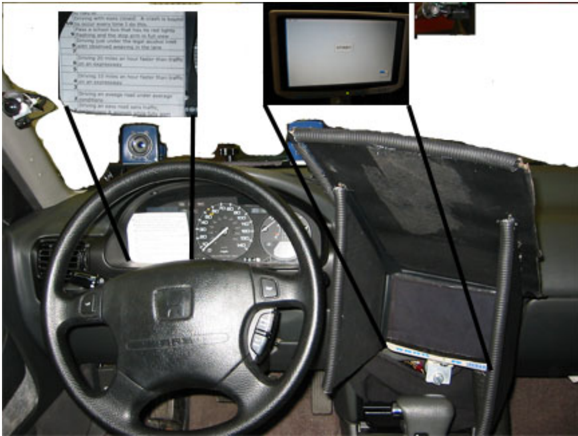
Figure 3.29. Dash layout with eye tracking system, risk rating sheet, and touch screen
