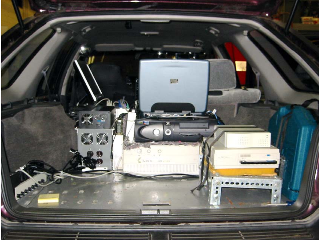
Figure 3.27. Honda Accord wagon cargo area showing (left to right) custom individually fused/switched power strips, DC/AC and DC/DC inverter, custom signal conditioner, headway sensor signal conditioner, Gateway 486 PC, Dell 310 PC, HP Pavilion laptop, external hard drive and Bernoulli, and blue tool box with road tools
