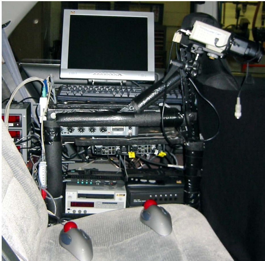
Figure 3.28. Rear seat equipment rack housing (bottom to top, left to right): Sony DSR-20 MD digital video recorder, RealTime QS21 Color Quad Splits, Tview, ViewSonic VB50HR TV tuner, Panasonic GP-KS152 controllers, Shure M267 mic mixer, IOGEAR 4 port KVM, main keyboard, ViewSonic VE510+ monitor, Logitech Marble Mouse (foreground)
