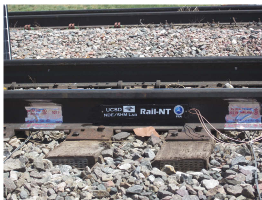
Testing of University of California-San Diego's rail neutral temperature measurement device on continuous welded rail with concrete ties at Transportation Technology Center, Inc. Note the strain gauge on each side for validation and comparison.
