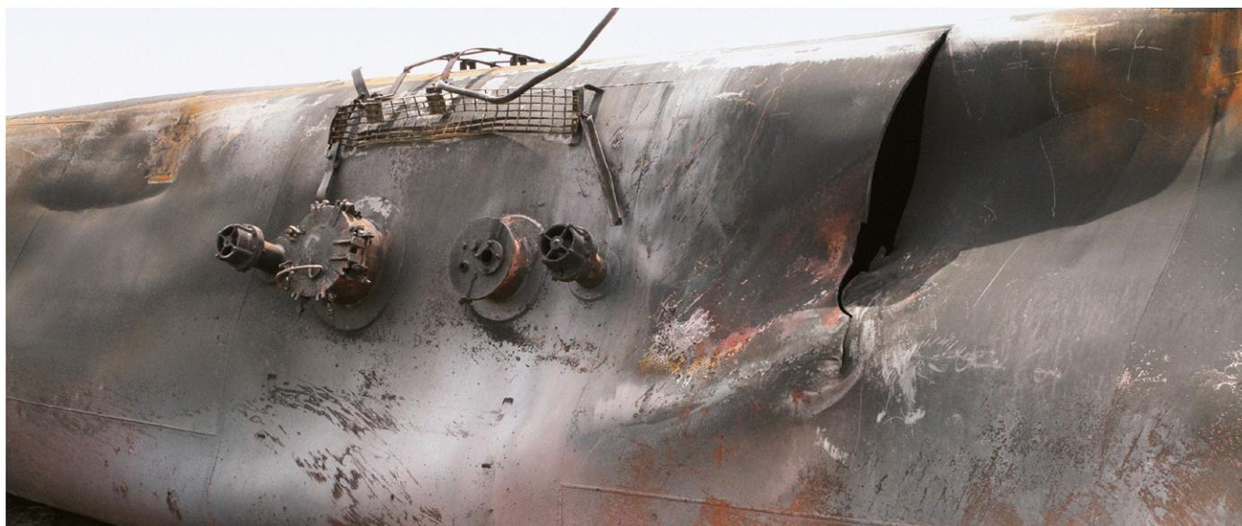
Tank car shell puncture from the Lac-Mégantic, Quebec, rail disaster in July 2013. Source: NTSB
