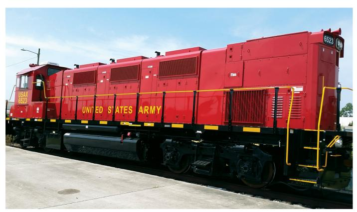
Pictured is an Ultra-Low Emitting Locomotive-U.S. Army locomotive USAX 6523 source: U.S. Army
