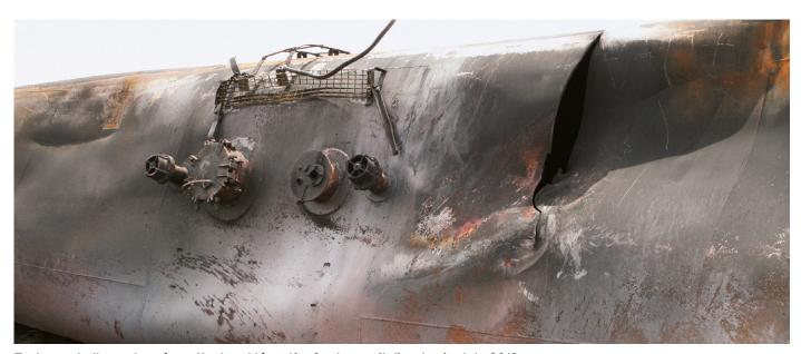
Tank car shell puncture from the Lac-Mégantic, Quebec, rail disaster in July 2013. Source: NTSB
