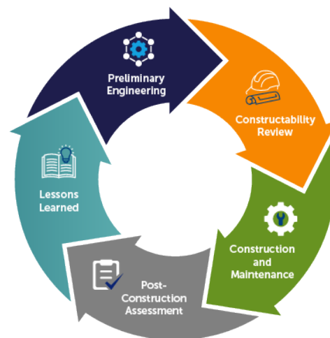
Figure 4: Incorporate constructability reviews and PCAs into the project delivery lifecycle.
