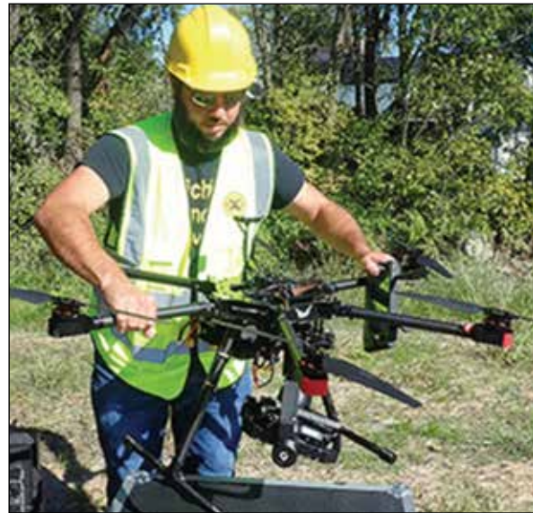
A MTRI technician prepares to launch a drone for a highway-rail grade crossing inspection. (Source: MTRI, Inc.)
