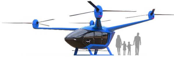
Figure 1: NASA RVL T quadrotor reference vehicle configuration considered in this study.
